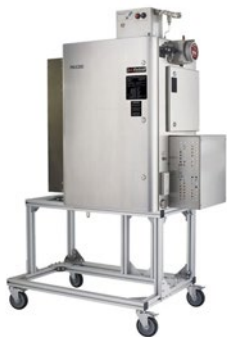
MAX300-BIO Real-Time, Multi-Stream, Industrial Mass Spectrometer for Bioreactor Control
