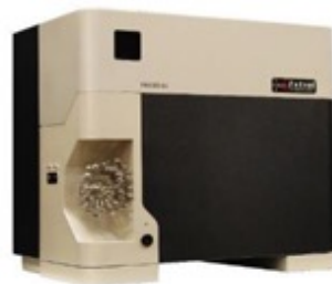
MAX300-LG Benchtop Mass Spectrometer for Real-Time, Multi-Stream, Bioreactor Control
