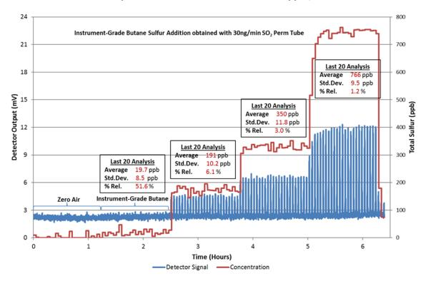
TraceS-1000 Linearity for Concentrations less than 1ppm/vol. in Butane
