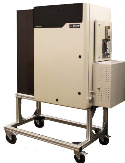
Figure 5. The MAX300-RTG, real-time mass spectrometer. For refinery flare compliance, the analyzer is often configured with a Hazardous Area Certification and corrosive-resistant materials that perform well with high-level H 2 S and HF acid, according to site requirements.
