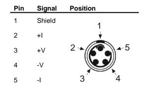
When the 5-pin LEMO connector is properly assembled, you will notice that the red dot of the connector housing will be aligned at the top directly above pin 1.
