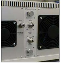
The input and output connectors are clearly labeled on the Sample Gas section of the back panel. Depending on the specific model and ordered options, the stainless steel gas input and output connections may be 6 mm Swagelok, <sup>1</sup>/<sub>4</sub> inch Swagelok, or <sup>1</sup>/<sub>4</sub> inch Cajon VCR.
