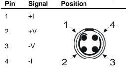
When the 4-pin LEMO connector is properly assembled, you will notice that the red dot of the connector housing will be aligned at the top between pins 1 and 4.
