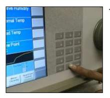
1. Press and hold the *enter* key on the numeric keypad for 3 or 4 seconds. If you've done it correctly, you'll hear two loud short beeps. If not, release the key and try again.
