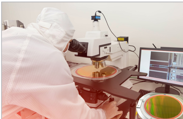
Fig. 1 Technician inspecting a silicon test wafer for potential damage
