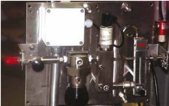
Typical sample system for measuring at atmospheric pressure.
