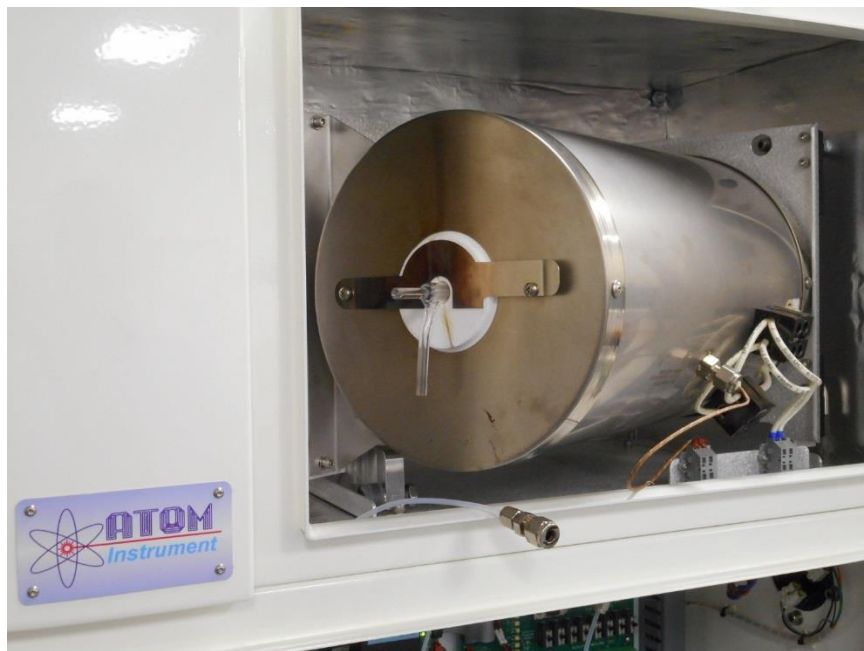
Above picture shows all fittings detached from the combustion tube.
