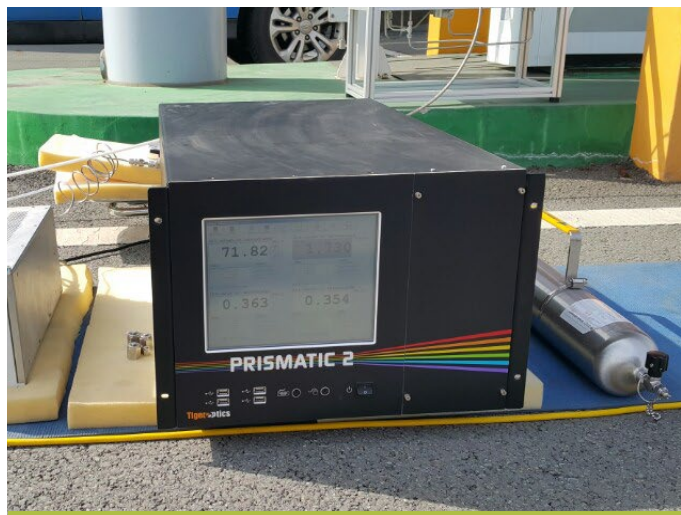
Fig. 2 Prismatic 2 at a hydrogen fueling station in South Korea (picture courtesy of Sunwoo Engineering)
